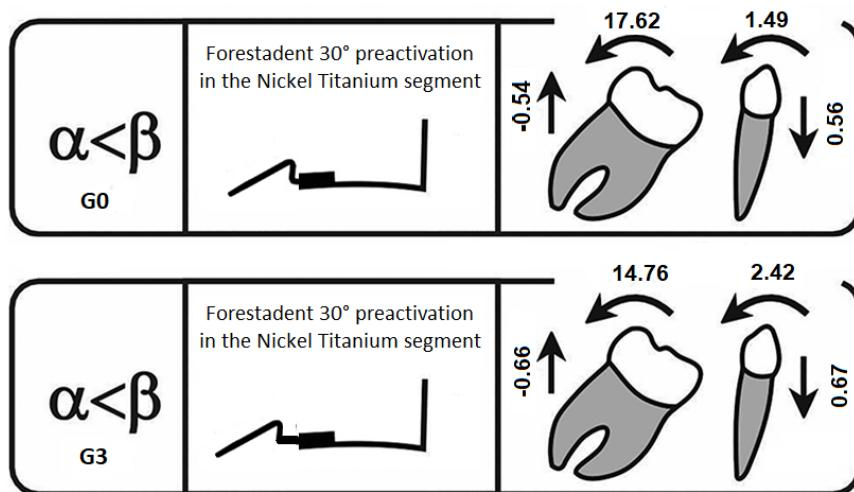
Vector illustration of the resulting mechanical systems: the arrows indicate the direction of vertical forces (\$Fz\$) and distal moments (\$Ty\$), demonstrating the consistency between experimental results and the theoretical Burstone Class III geometry<sup>8888</sup>. **Source:** Adapted from Wichelhaus and Sander (1995).
