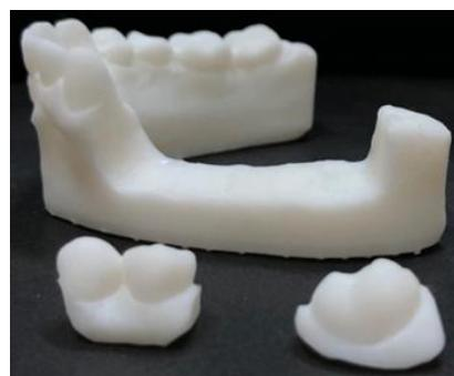
High-resolution 3D printing of the segmented dental crowns (first premolar, second premolar, and second molar), designed to be attached independently to the load cells of the Orthodontic Force Tester (OFT) for precise force recording.
