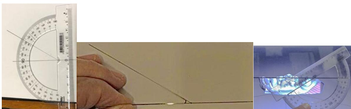
The standardization of the model involved (1A) the customized protractor template, (1B) the physical check of the 30° mesial inclination on the laboratory bench, and (1C) the digital confirmation of the molar position relative to the occlusal plane using Meshmixer software.
