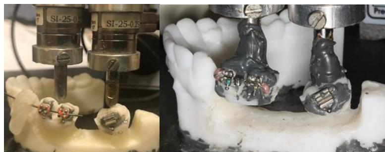
Detailed view of the Nano17 sensors: (A) strategic positioning of the T1 sensor between the premolars and T2 on the molar; (B) final fixation with epoxy glue and removal of the wax to allow unrestricted 3D measurement of forces and moments.
