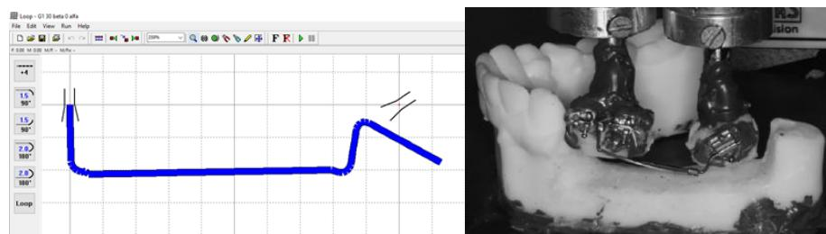
(A) The MTS design template within the Loop software environment for standardized geometry; (B) Clinical simulation showing the Memory Titanol Spring (MTS) activated and connected to the transducer system.
