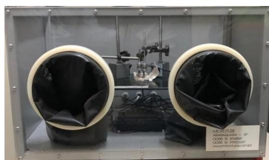
The testing apparatus was housed in an acrylic glove box equipped with a heating system maintained at a constant temperature of 37°C, essential for evaluating the superelastic properties of the nickel-titanium alloy under clinical-like conditions.
