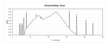
Note that in figure 5 there are some spikes on the deep drawing profile, that is some noises generated during the deep drawing operation.
