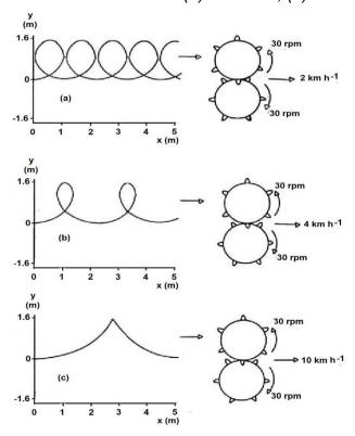
Angular velocity = 30 rpm, peripheral velocity = 9 km h-1
