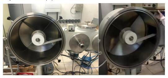
Can be possible to deposit meters of filters at once, which makes the process faster, in addition to being a simple and economical process. Once the vacuum is established, successive depositions can be made on the entire inserted roll.
