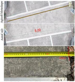
On-site (reference values) using a metal tape measure
