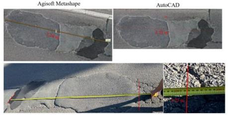
On site (reference values) using a metal tape measure
