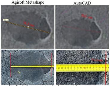
On site (reference values) using a metal tape measure
