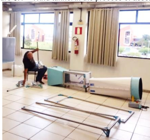
Figure 3.1 – Wind tunnel in the process of assembly
