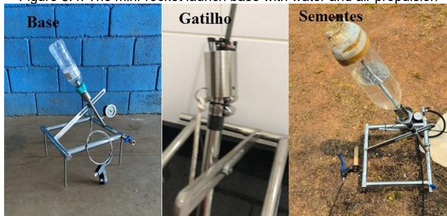
Figure 3.4. The mini-rocket launch base with water and air propulsion
