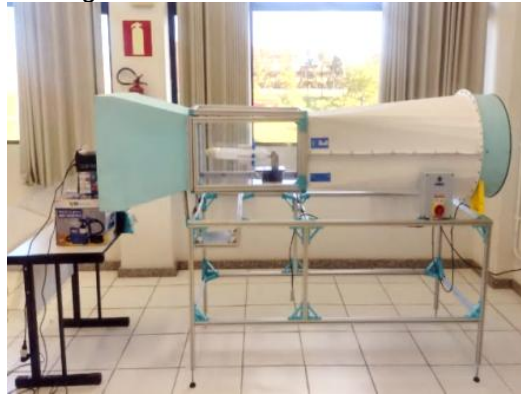
Figure 3.7 – Assembled vent tunnel
