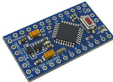
Figure 4: Representative image of an embedded board of the Arduino Pro Mini model of 5 volts and 16MHz.
