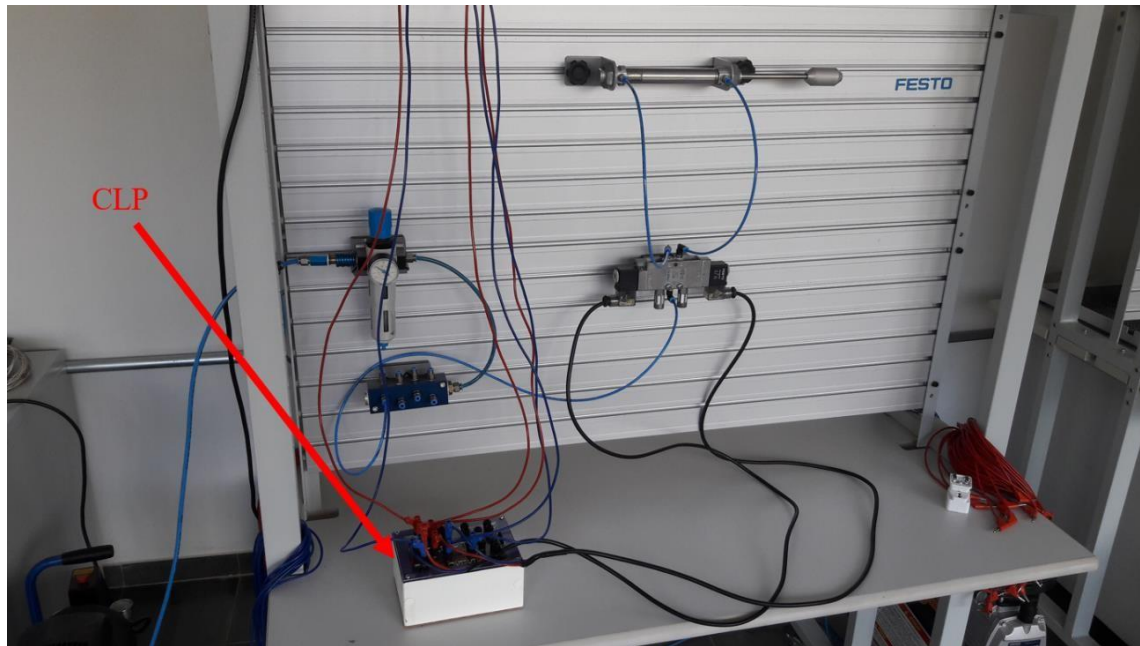
Figure 23: Image of the PLC in operation on the pneumatics bench of the mechanics laboratory of UFVJM.
