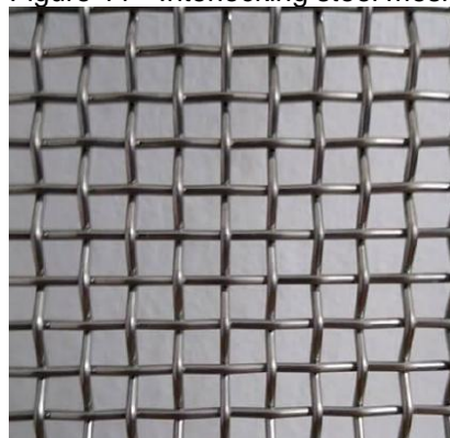
Figure 11 - Interlocking steel mesh
