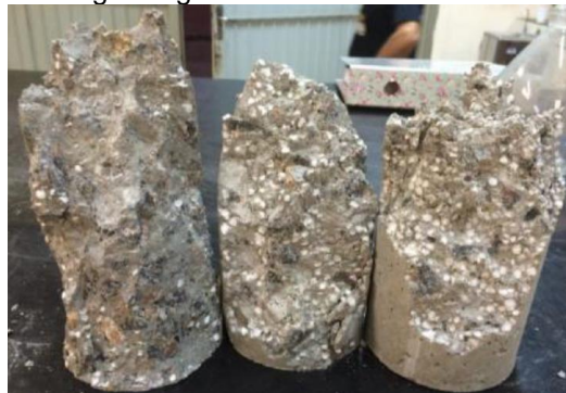
Figure 7 Lightweight concrete made with EPS beads
