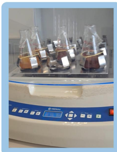
Figure 16: Oil in the shaker for agitation and homogenization of the sample.
