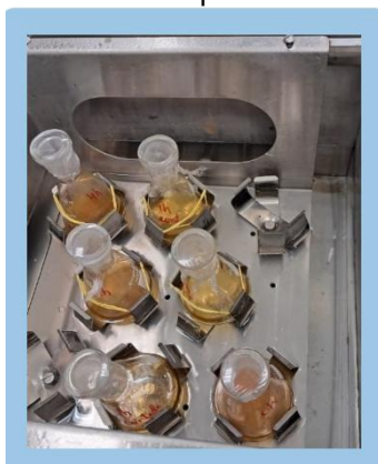
Figure 9: Samples during the incubation period in a thermostated bath at 35°C.
