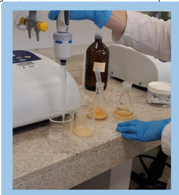
Figure 6: Addition of ethanol acetone to the oily fraction
