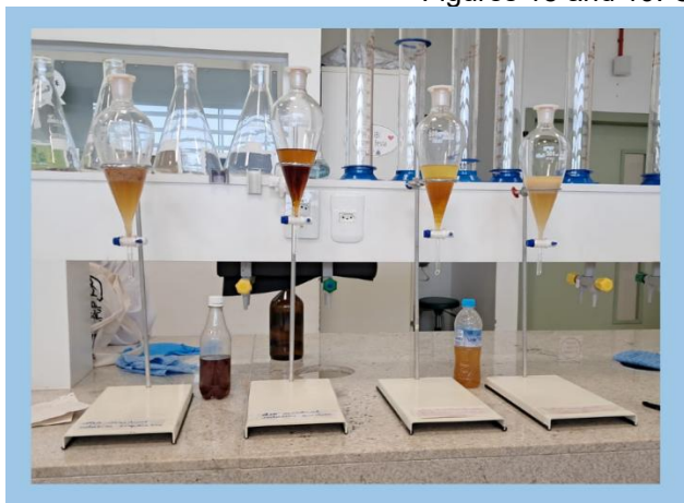
Figures 18 and 19: Oil in the settling funnel.
