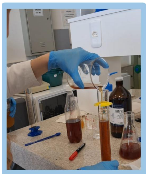
Figure 14: Measurement of the oily fraction , showing the process of quantification of the volume of oil present in the sample
