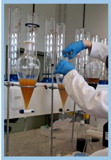
Figure 17: Transfer of the oil to the settling hopper.
