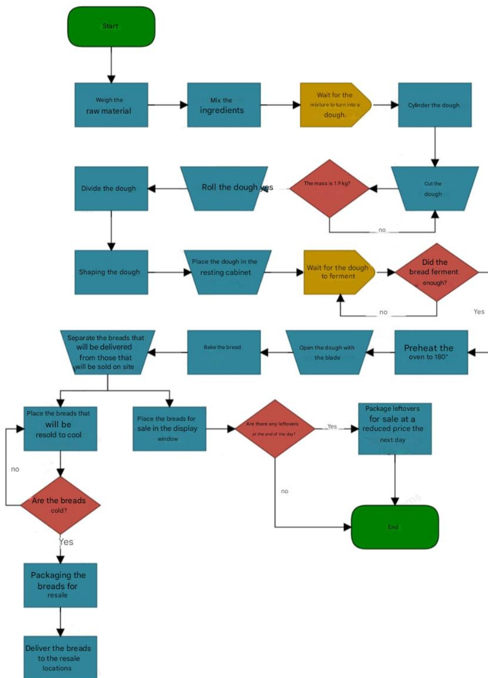
Figure 2 - Flowchart of the French bread production process
