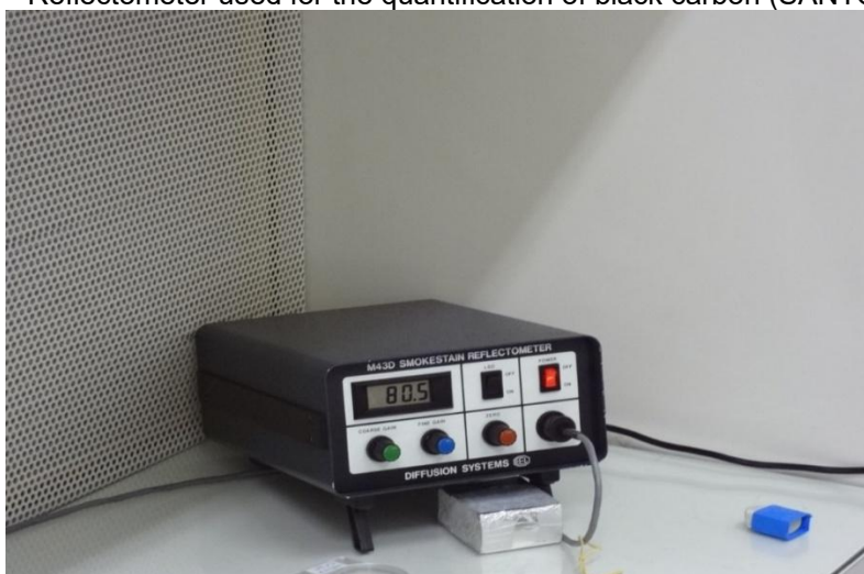
Figure 4 – Reflectometer used for the quantification of black carbon (SANTOS, 2014).
