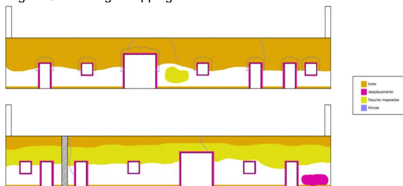
Figure 3 – Damage mapping on the E1 and E2 facades of the Station
