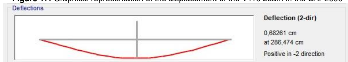
Figure 17: Graphical representation of the displacement of the V116 beam in the SAP2000
