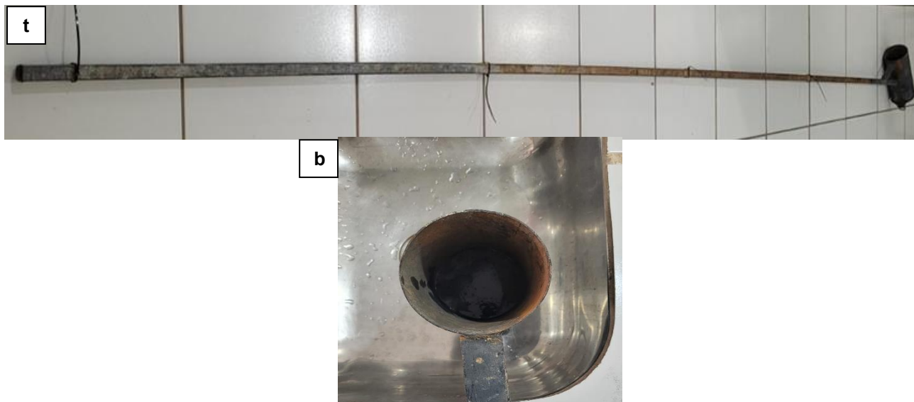
Figure 4 – Instruments used for field collections: a) sediment collector; b) Aluminum container for collection for substrate.
