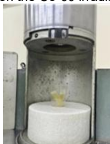
Figure 3. Samples on the Co-60 irradiator - GamaCell 220.
