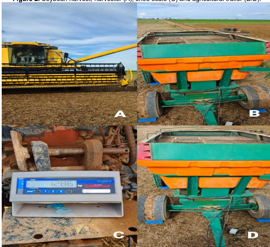
Figure 2. Soybean harvest, harvester (A); shoe scale (C) and agricultural trailer (B/D).
