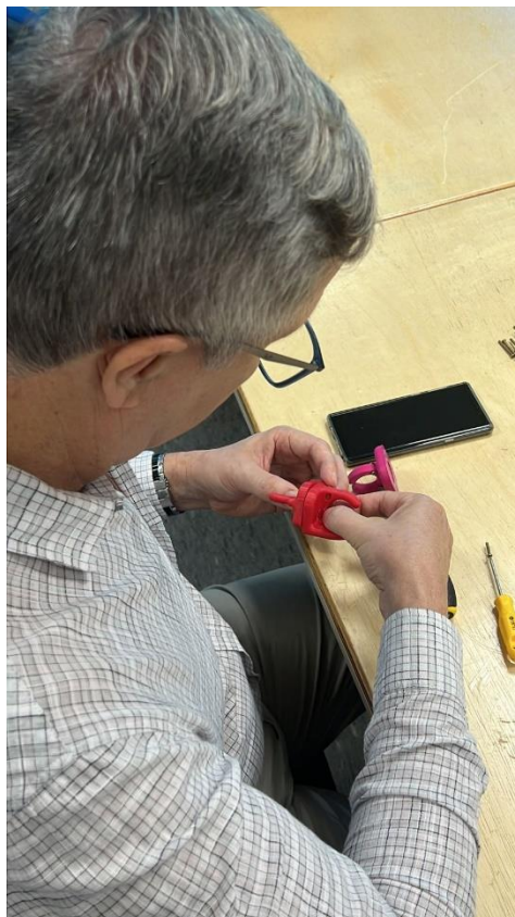
Fig. 13 – a prototype of the muletas support being assembled after printing on a 3D printer, from the Maker Laboratory
