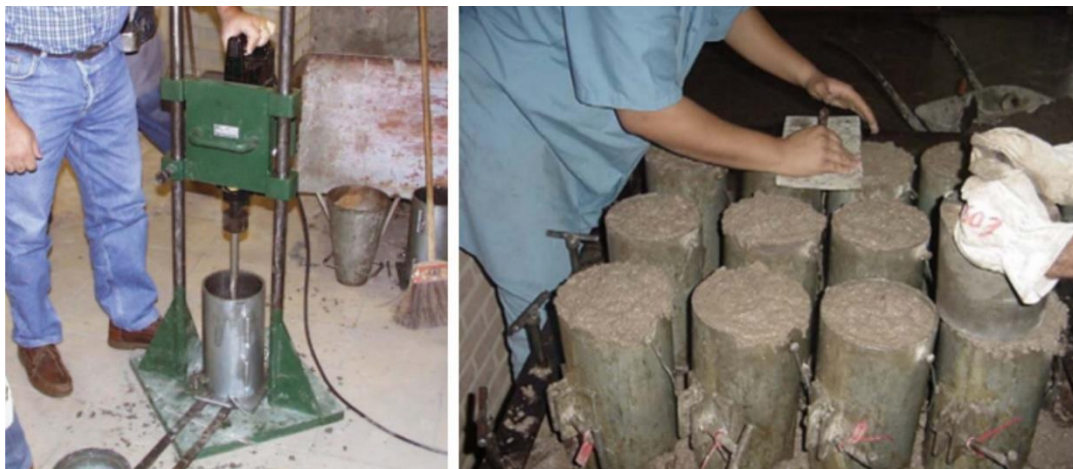
Figure 2. On the left: thickening of the specimen with a Kango Type Hammer; Right: Dense specimens on a vibrating table.
