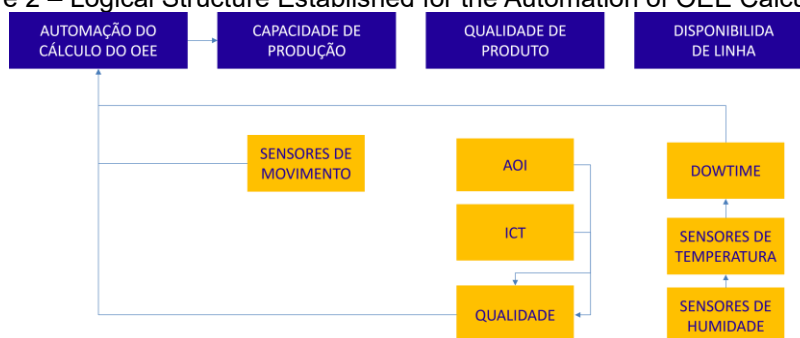
Figure 2 – Logical Structure Established for the Automation of OEE Calculation.
