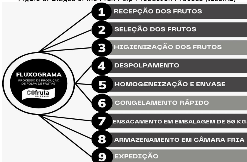
Figure 8: Stages of the Fruit Pulp Production Process (tucumã)
