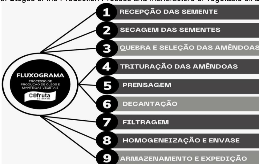
Figure 9: Stages of the Production Process and manufacture of vegetable oil and butter
