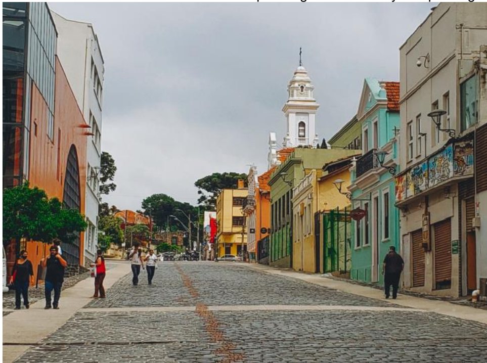
FIGURE 8: In the photograph, Dr. Claudino dos Santos Street, which gives access to Largo da Ordem itself, with the implementation of a 1.5-meter-wide concrete strip aiming at accessibility and painting of the facades.
