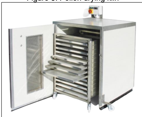
Figure 3. Pollen drying kiln
