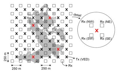
As the campaign sampled several points outside of Marlim, the VVCSEM response in each quadrant where the reading was taken above the reservoir will be shown here. Each quadrant was named Q1, Q2, Q3, and Q4 from left to right and bottom to top. The Marlim model has a bathymetric range of 105 m to 1513 m, so the length of the VED was variable at each reading point so that Q1 is 800 m, Q2 is 1210 m, Q3 is 400 m, and Q4 is 210 m.
