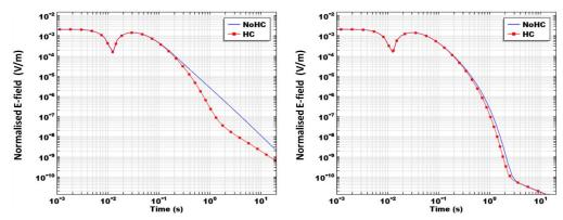
Unlike the MCSEM response, the VVCSEM response exhibits the curve representing the environment's response with a reservoir (HC) below the curve of the environment without the reservoir (NoHC). This signature has the same characteristics as the other transient methods since a lousy conductor (resistive) tends to promote a faster electromagnetic field decay. Thus, the presence of the reservoir is perceptible when the HC curve is compared with the background curve.
