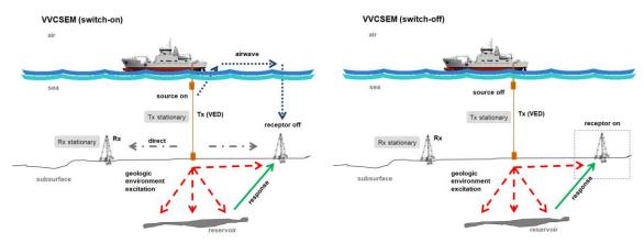
For analysis of the collected data, a comparison is made of the responses in environments (or models) with no hydrocarbons (NoHC)  $E_0(t)$  and compared with the presence of hydrocarbons (HC)  $E_{HC}(t)$ ; thus, the anomalous vertical field is:
