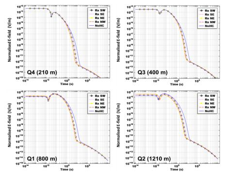
As expected, the VVCSEM response in the MR3DC model is very similar to that in the canonical model with the insertion of the saline layer. The particularity of the Marlim is that it is anisotropic; each measurement point reflects a different organisation of the geological environment (bathymetry, thickness, depth, and physical property of each stratum).
