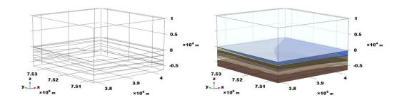
In the construction of the model, in addition to importing and interpolating the horizons, the horizons had to be converted into solids and interposed in a larger enclosing block, which was later trimmed with the horizon limits. To simplify the nomenclature, the Marlim model built in the multiphysics modeller will be called MR3DC.
