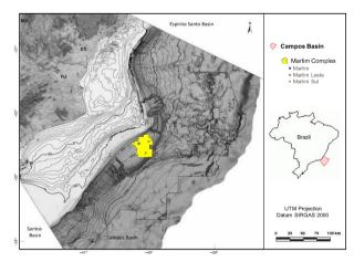
The region of the Campos Basin where the Marlim Field is located has a challenging bathymetry from the perspective of collecting data with vertical dipoles since it is difficult to maintain the verticalisation of the source, and there is, in many cases, a significant difference in elevation between the source and the receivers depending on the offset.
