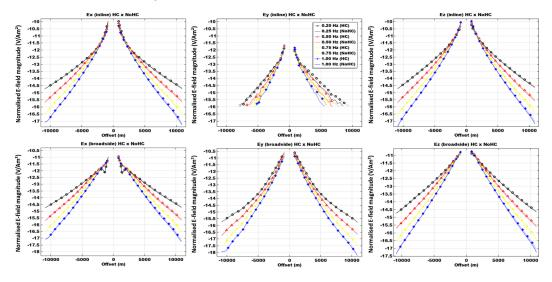
The MCSEM result on MR3DC shows the reservoir response to be relatively weak due to the thick and highly resistive salt layer in the Albian. The responses of the  $E_x$ ,  $E_y$ , and  $E_z$  components are very similar in the inline and broadside, except for the curves presented in  $E_y$  (inline), where the difference between the background (NoHC) and reservoir (HC) curves is more significant but distorted.
