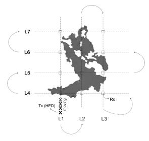
The acquisition lines (L1-L4) are 10 km long each, and the result will be displayed graphically using plot group 1D. The response for the  $E_x$ ,  $E_y$ , and  $E_z$  field components inline
