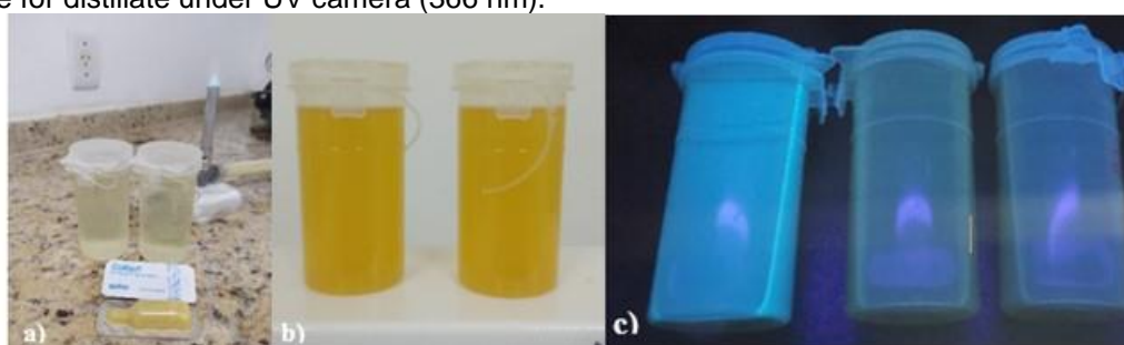
Figure 7. P/A test for identification of total coliforms and Escherichia coli from the raw and distilled sample. (a) the test for P/A was inserted. (b) positive for total coliforms (c) positive for Escherichia coli in the raw sample and negative for distillate under UV camera (366 nm).
