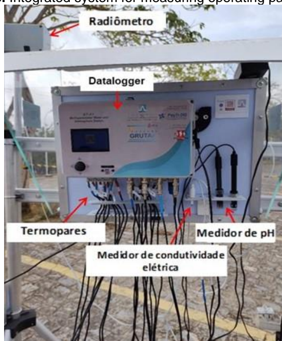
Figure 3. Integrated system for measuring operating parameters.
