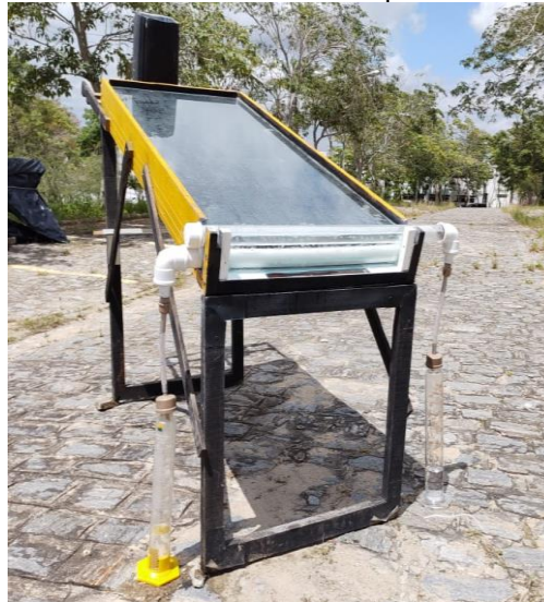
Figure 1. Solar Distiller with Wave Shape Heat Absorber Plate
