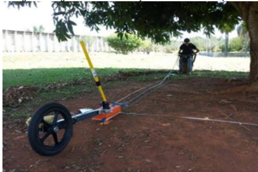
Fig. 6. Arrangement of the GPR System used in data acquisition.
