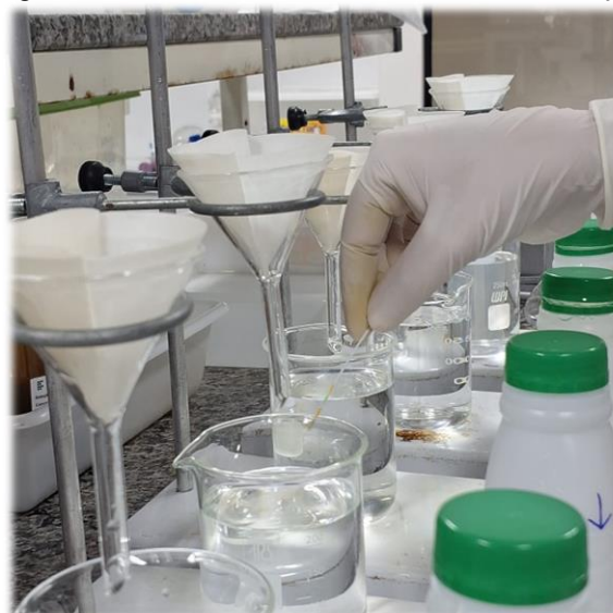
Figure 5 – Filtration and measurement of water pH
