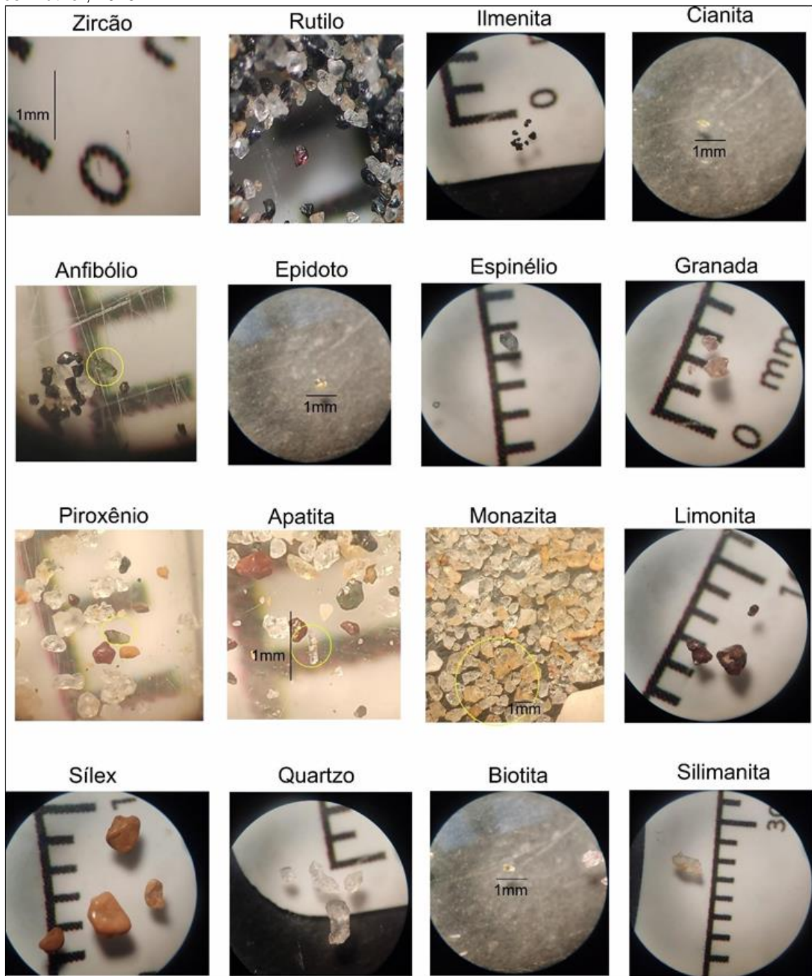
Figure 12: Photo of the minerals identified by means of the magnifying glass in the sedimentology laboratory. Source: Author, 2023.
