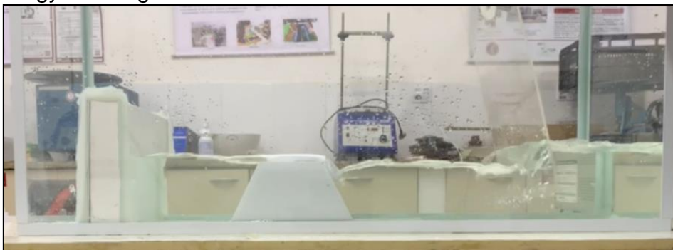
Photo: Experiment/Model Láb. Civil Engineer – UniVassouras/RJ, Submerged Breakwater Slope with energy stacking
