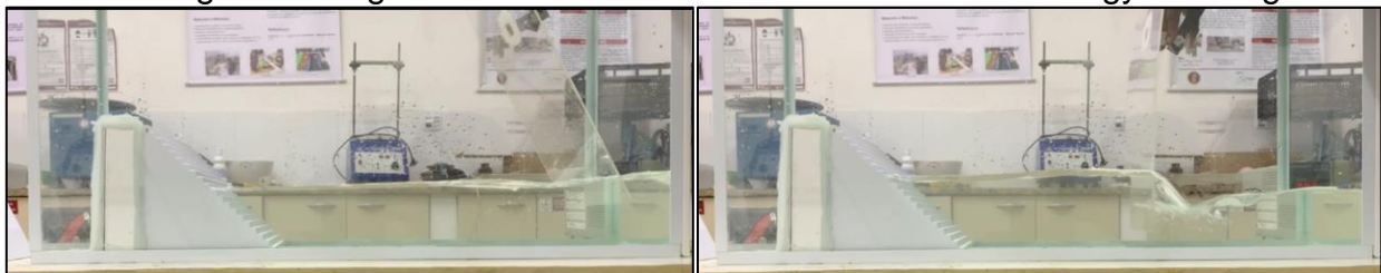
Photos: Experiment/Model Láb. Civil Engineer – UniVassouras/RJ, Slope Staggered and inclined coating with elongated wave in formation and with wave to energy stacking
