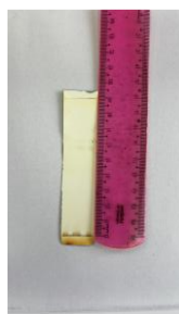
Figure 03: Samples eluted on the chromatographic plate revealed by iodine with respective rf values of the samples: leaf extracts by the static method with ethanol solvent, leaf by the ethanol ultrasound method and leaf by the ethanol soxhlet method. Rf 1: 0.6 and Rf 2 = 0.72 Rf 3 = 0.74.
