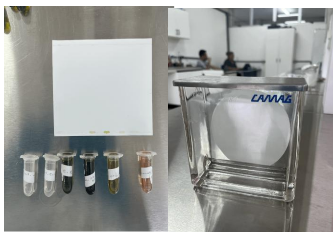
Figure 02: A: Samples that were applied to the thin layer chromatography plate B: Chromatographic tank prepared and saturated for elution.
