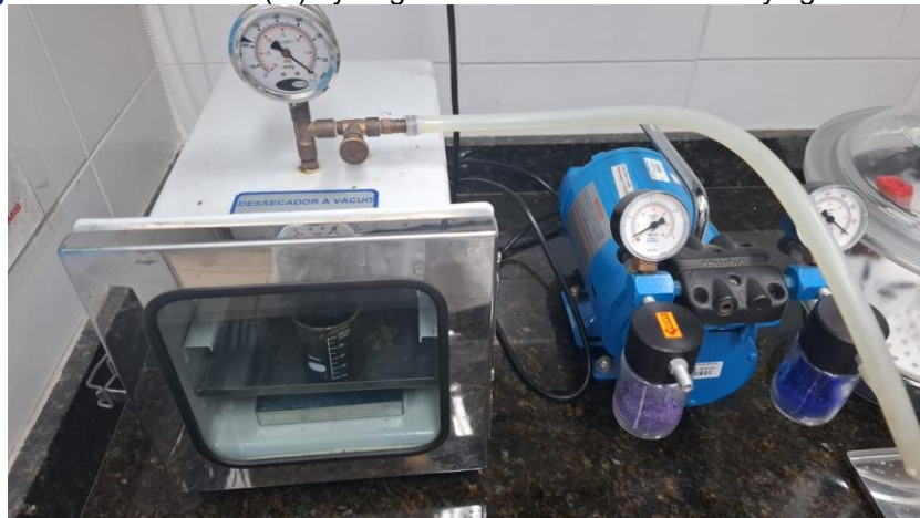
Figure 5 - Chitosan-Fe(III) hydrogel and carbon in vacuum drying oven at 300
