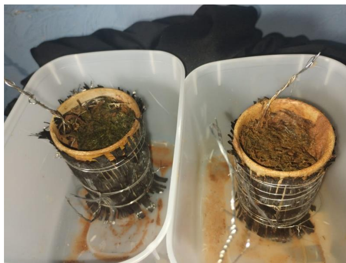
Figure 17 - BCMs from left to right, conventional gas diffuser layer, gas diffuser layer with Fe-N-C hydrogel catalyst
