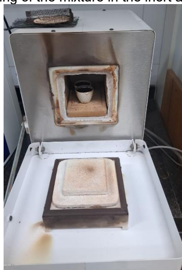
Figure 6 - Heating of the mixture in the inert atmosphere oven.
