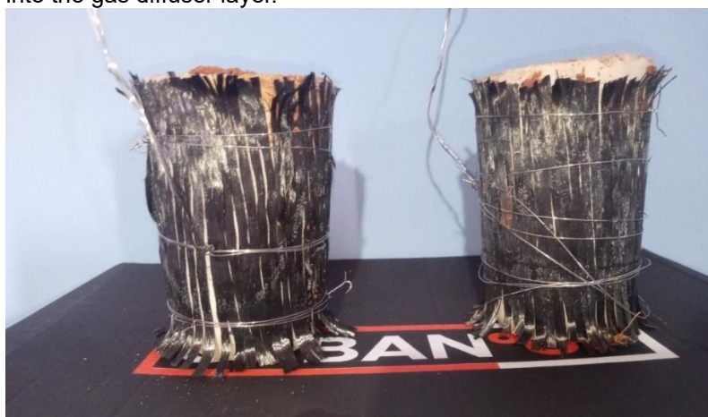
Figure 8 - Cathode already inserted in the BCMs, from left to right: gas diffuser layer and Fe-N-C hydrogel catalyst incorporated into the gas diffuser layer.
