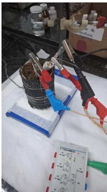
Figure 10 – Experiments in half cell for developed electrochemical cell. The anode as the working electrode, a platinum plate as the counter electrode, and an Ag/AgCl reference electrode were used for the potential measurements.
