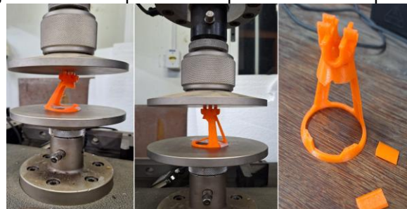
Figure 12 – Test specimens ruptured under compression
