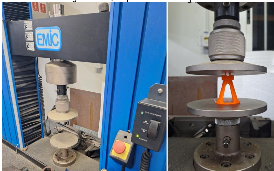
Figure 11 – Compression test of spacers
