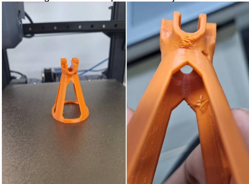
Figure 7 – ABS spacer after adjustments.
