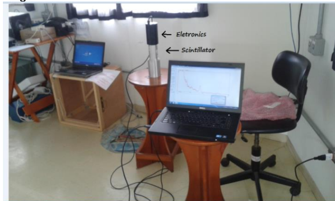
Fig. 1: View of gamma scintillator with associated electronics and computer. (Autor)
